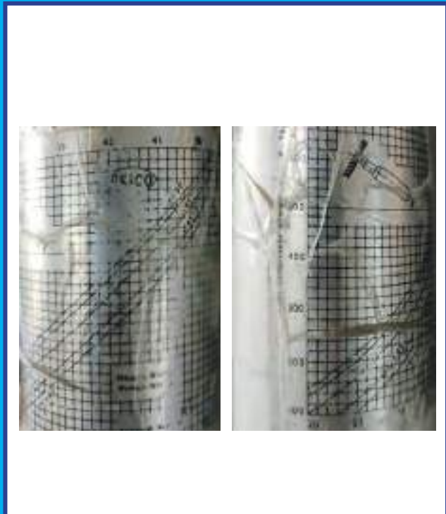
Curve between rebound number and compressive strength for various alignment of rebound hammer.
